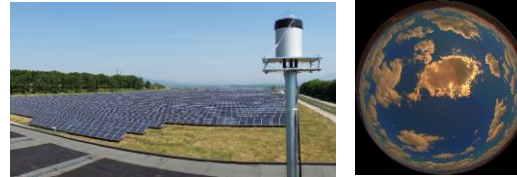
Cloud tracking – prediction of the power output from a solar PV park
